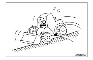
The engine angularity limits are 30°. Do not operate by more than the engine limits in any case.
